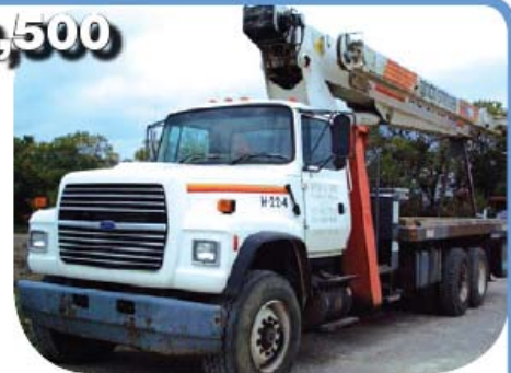
1997 Terex 4485 22 ton on Ford F8000 w/tag axle 85'-95' main w/40' jib, Cummins eng, ~83,000 mi.
